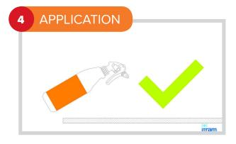
Apply at approx 45° angle and within 15cm from surface in solid stream.
