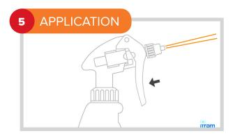
Pump smoothly and gently to ensure solid stream, do not atomise. Aim to cover 10cm<sup>2</sup> area.
