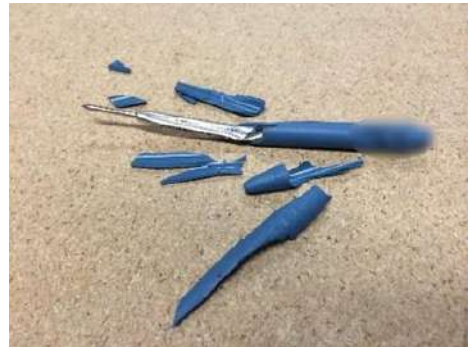
Low quality detectable plastics can increase foreign body risks Image © BST Detectable Products
